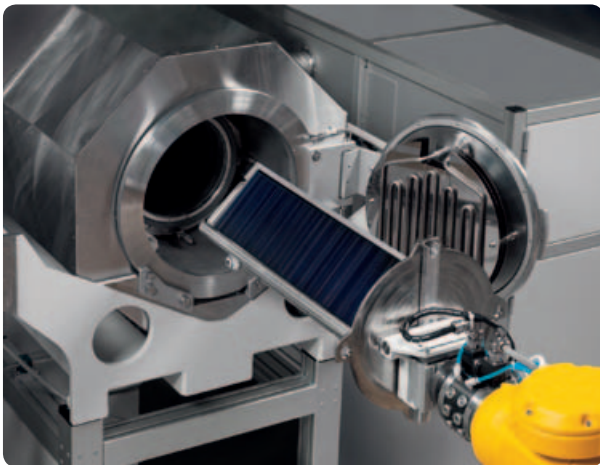
The TFS NX300, a fully automated multiple ALD coating system for strengthening glass or surface passivation of crystalline silicon solar cells.
