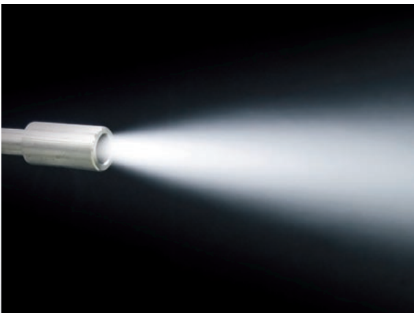
nAERO process produces an aerosol with submicron droplet size.
