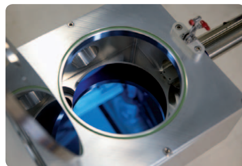
TFS 200 load lock with substrate inside.
